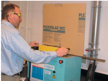
Automatic edge finishing machine with a diamond-tipped spindle smooths saw cut, producing a fine and glossy edge to Plexiglas® acrylic sheet.
