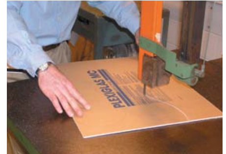
Use band saws for rough cutting larger-radius curves or for making rough straight cuts in thick sheet.
